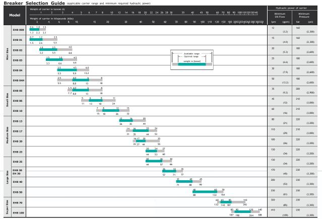
This guide is valid for the normal excavators equipped with standard boom-arm. For carriers with special features, contact your Everdigm dealer or service.
